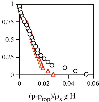
Fig. 2. Comparison of vertical profiles of dimensionless pressure in simulated “atmospheric” (O) and “pressurized” tests (Δ) with  $Fr = 168$  and  $M/R = 0.0052$ . The “atmospheric” conditions are  $L = 1220$ ,  $Ar = 46$ ,  $R = 4860$  and  $M = 26$ ; the “pressurized” conditions are  $L = 1410$ ,  $Ar = 554$ ,  $R = 407$  and  $M = 2.1$ .
