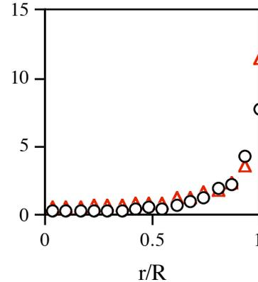
Fig. 3. Profiles of particle volume fraction versus relative radial distance at the elevation  $z/H = 0.5$ . By symmetry, only one side is shown. For conditions and symbols, see Fig. 2.
