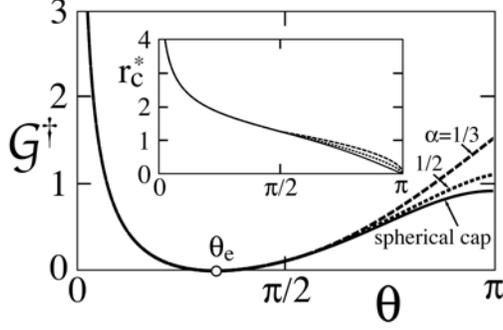
Figure 3: Interface potential energy  $\mathcal{G}^\dagger$  vs  $\theta$  for  $\theta_e = \pi/3$ . Inset: dimensionless contact patch radius  $r_c^*$  vs  $\theta$ . Solid, dashed and dotted lines represent, respectively, expressions for a spherical cap,<sup>11</sup> and corrections consistent with  $\alpha = 1/2$  and  $1/3$ , respectively.
